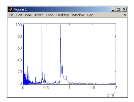
**3** Normalize the ion intensity of every spectrum to the maximum intensity of the single highest peak from any of the spectra in the range above 100 m/z.
