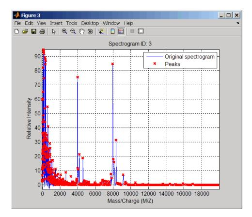
**6** Use the cellfun function to remove all peaks with m/z values less than 2000 from the eight peaks lists in output P. Then plot the peaks of the third spectrum (in red) over its smoothed signal (in blue).
