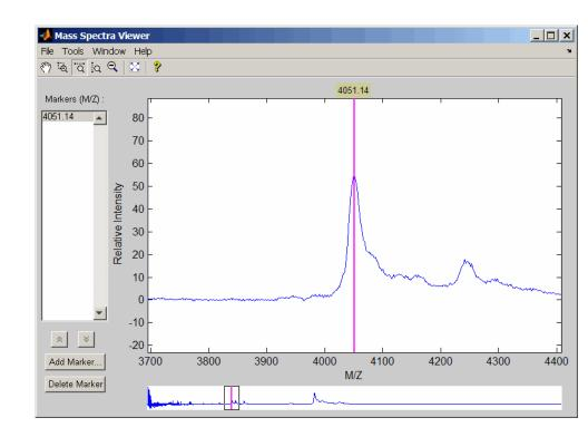
**3** Shift a spectrum by the difference between RP, the known reference mass of 4000 m/z, and SP, the experimental mass of 4051.14 m/z.
