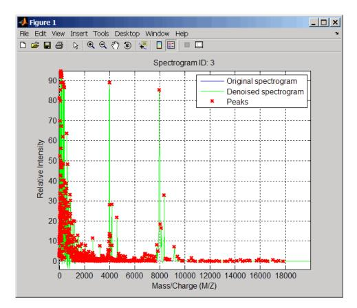
**5** Smooth the signal using the mslowess function. Then convert the smoothed data to a peak list by finding relevant peaks and plot the third spectrum.
