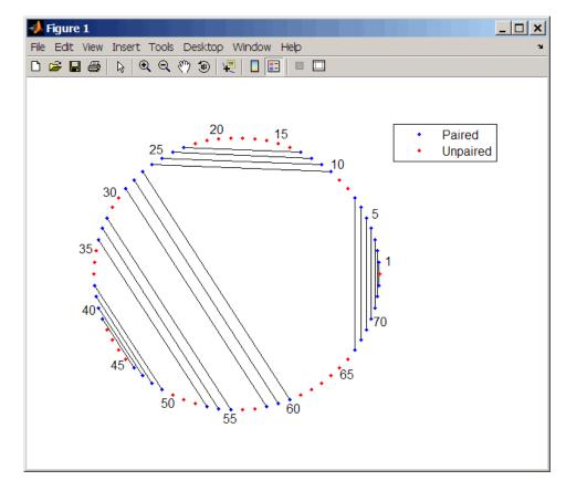
**2** Plot the RNA sequence secondary structure in graph format and color it by pair type.
