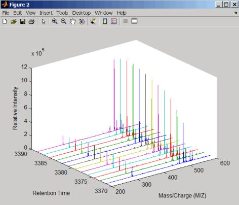
4 Resample the data to plot the Total Ion Chromatogram (TIC).
