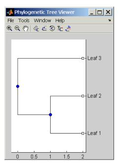
Tree = phytree(B, D) creates an additive (ultrametric or nonultrametric) phylogenetic tree object with branch distances defined by D. D is a numeric array of size [NUMNODES X 1] with the distances of every child node (leaf or branch) to its parent branch equal to NUMNODES = NUMLEAVES + NUMBRANCHES. The last distance in D is the distance of the root node and is meaningless.
