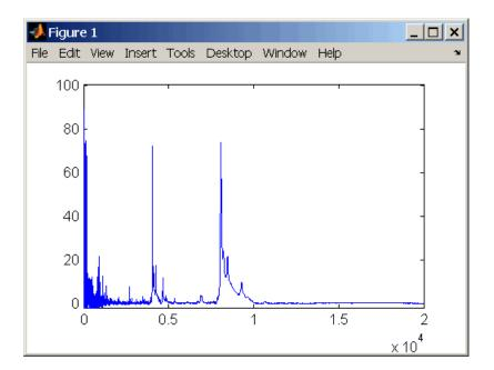
**2** Normalize the AUC of every spectrum to its median, eliminating low-mass noise, and post-rescaling such that the maximum intensity is 100.
